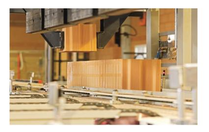
Based on given data the necessary amount of bricks is fed into the production line.
