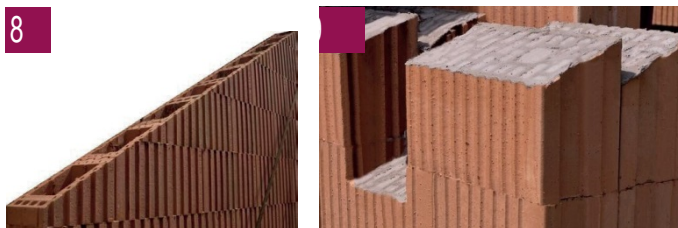
Image 8-9 • Required bevels are cut in the production hall with special cutting processes.
